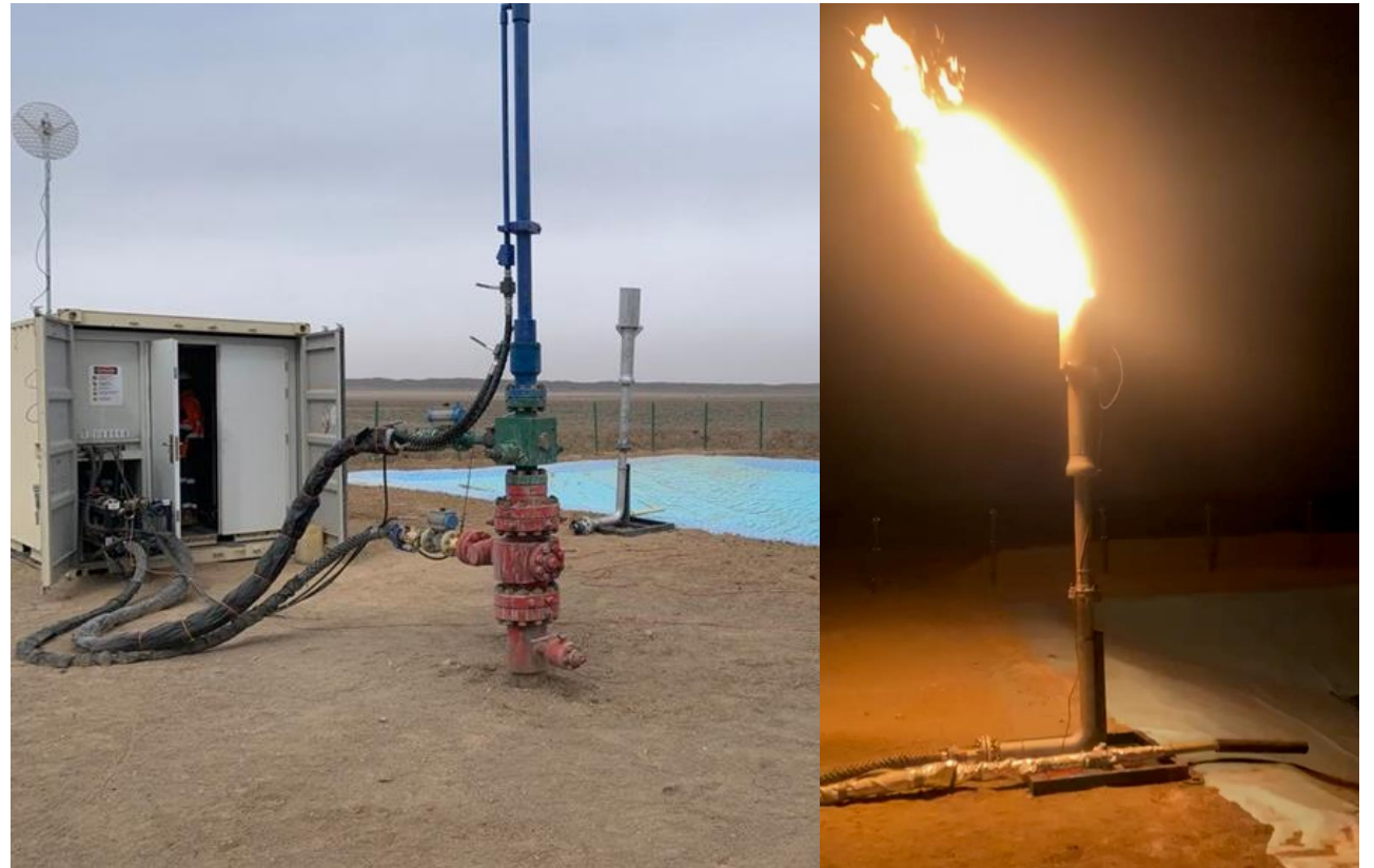
Extended testing equipment at Red Lake-7 and first flare at Red Lake-5
