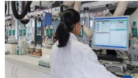
Early stage metallurgy. Weak acid (~ pH 4) leach testwork to determine level of REE hosted as ionic adsorption. Reject projects early which require difficult extraction
