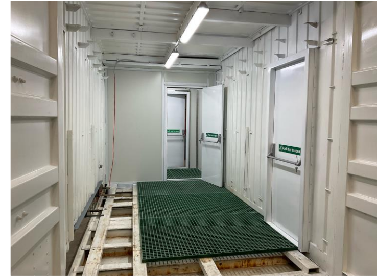
Wellhouse Container with bunding under fabrication
