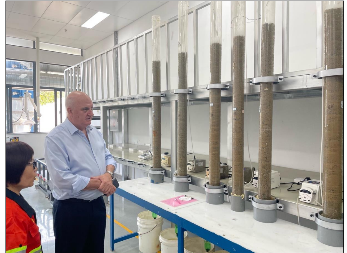
Oxide Column Leach at Zijin Research Labs
